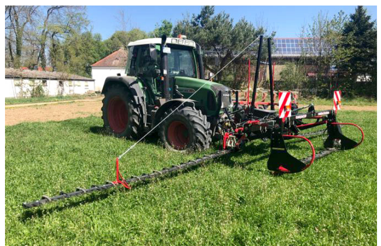
Mechanical weed control by tensioning the side cutting units
